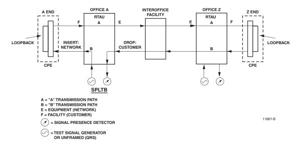
Figure 570-9. Typical Round-Robin Test Configuration
